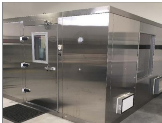
Figure 2: Stainless Steel Bioaerosol Test Chamber used for all Violet L Testing. The chamber is equipped with HEPA filtered air (in/out), multiple bio aerosol sampling ports, decontamination, and pressure balance. Exterior picture.
