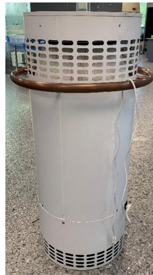
Figure 1: Violet L Device: The Violet L device is a standalone air purification system equipped with HEPA filtration and a photocatalytic vortex chamber that uses UV-C emitters. The pictured device has a prototype enclosure with production working components.
